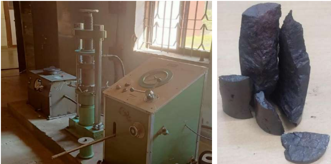
Fig VI: Triaxial Setup and Fractured Sample
