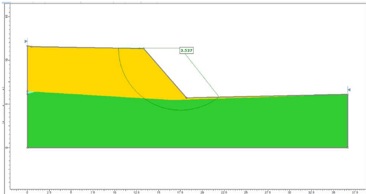
Figure 24 slope stability analysis of a laterite and shale slope showing FOS of 2.527
