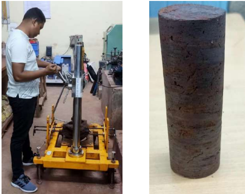
Figure IV. Coring operation and cored specimen
