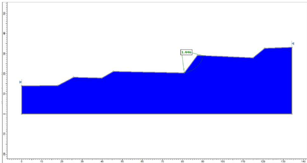
Figure 46 slope stability analysis of a friable ore slope showing FOS of 1.446
