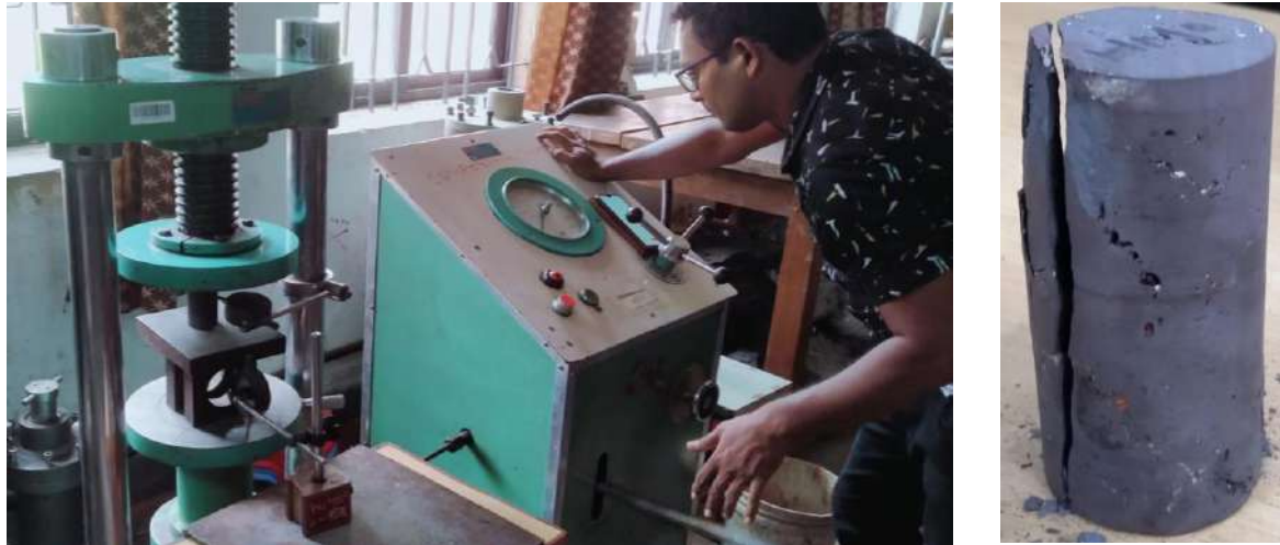
Figure V. Determining UCS of rock sample
