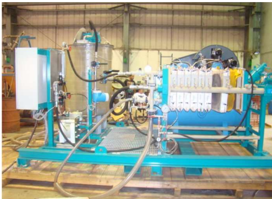
Fig. 2.9 Pilot scale pressure filter set up
