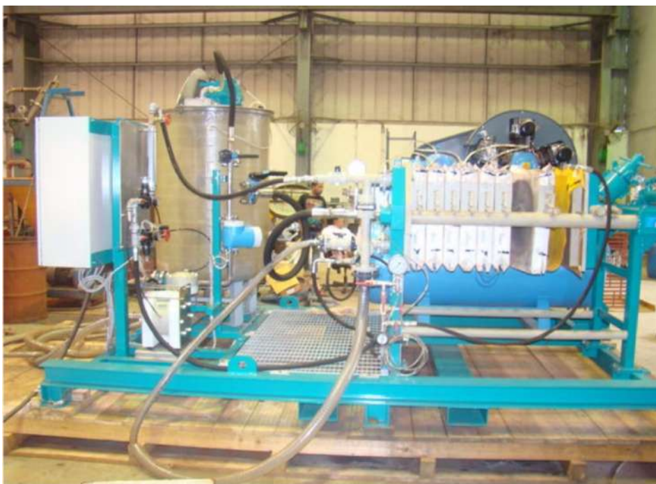
Fig. 3.8 Pilot scale pressure filter set up
